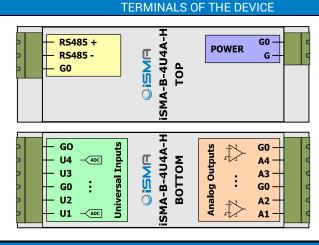
All G0 terminals are connected together internally
