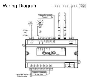
The FW-14 comes with one standard RS485 driver to support BACnet MSTP Client. The FW-14 also comes with two Ethernet Ports to program the Sedona Application, TCOM, FGP2P, BACnet and for web configurations.
