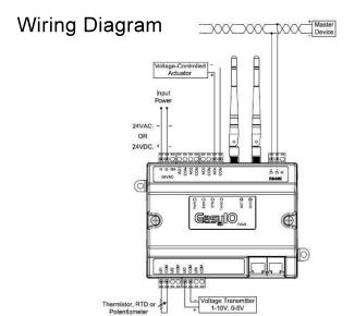
The FW-8 comes with one standard RS485 driver to support BACnet MSTP. The FW-8 also comes with two Ethernet Ports to program the Sedona Application, TCOM, FGP2P, BACnet and for web configurations.
