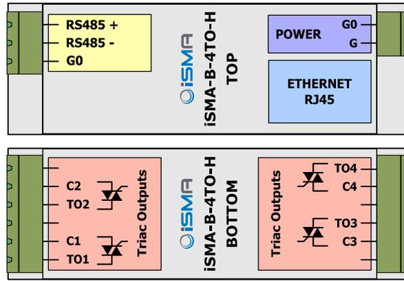
**All G0 terminals are connected together internally**
